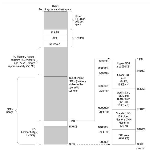
Figure 9. Detailed System Memory Address Map
